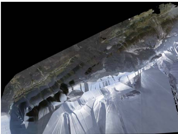
FIG. 53: The calculated orthophoto is not usable due to interfering background noise of the cloudy sky. (Source: own illustration)
