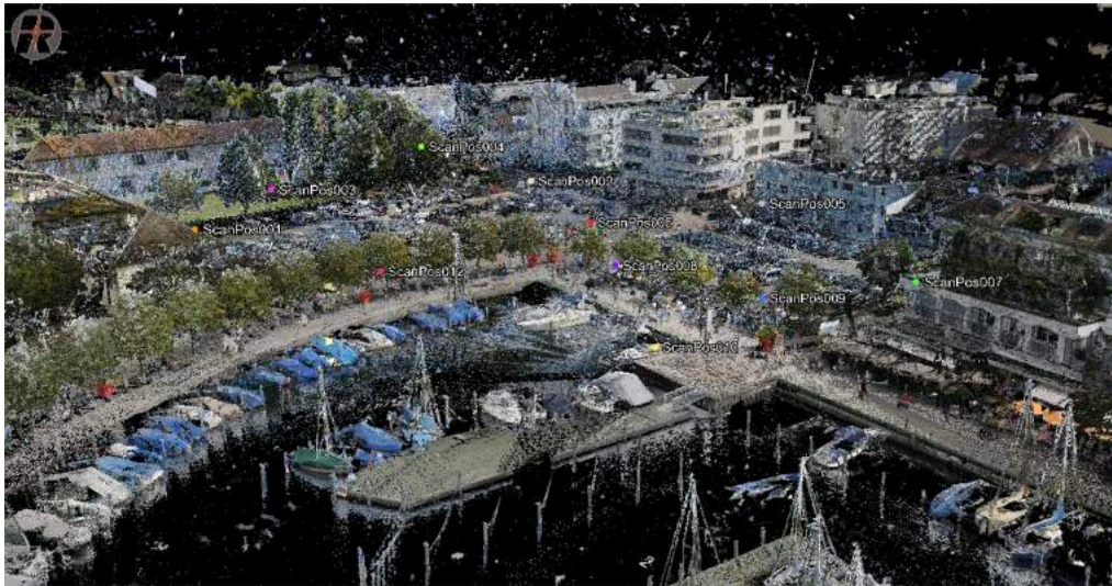
Figure 3.5: Noisy point cloud model of the Lachen harbour in RiSCAN Pro (RIEGL, 2014), with the car parks in the centre, the school area on the left, and the Octapharma area on the right
