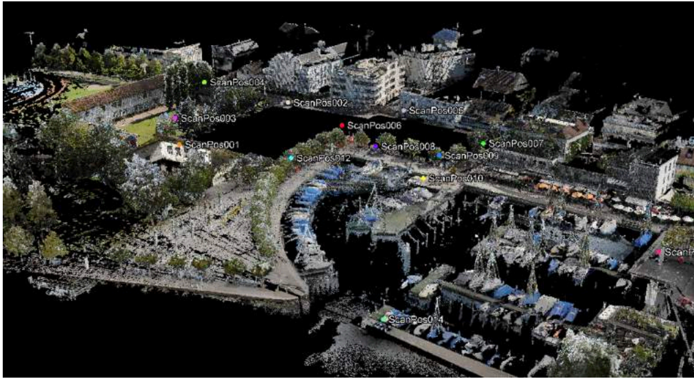
Figure 2.3: 3D point cloud model of the harbour area of Lachen in Switzerland
