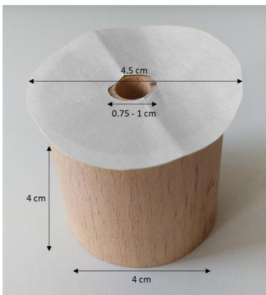
Fig. 9: Artificial flower used in acclimatisation cages: circular paper flowers with a diameter of 4.5 cm on wooden cylinders (4 cm x 4 cm) holding the Eppendorf tube (diameter of cavity: 0.75 cm, depth 1.3 cm).
