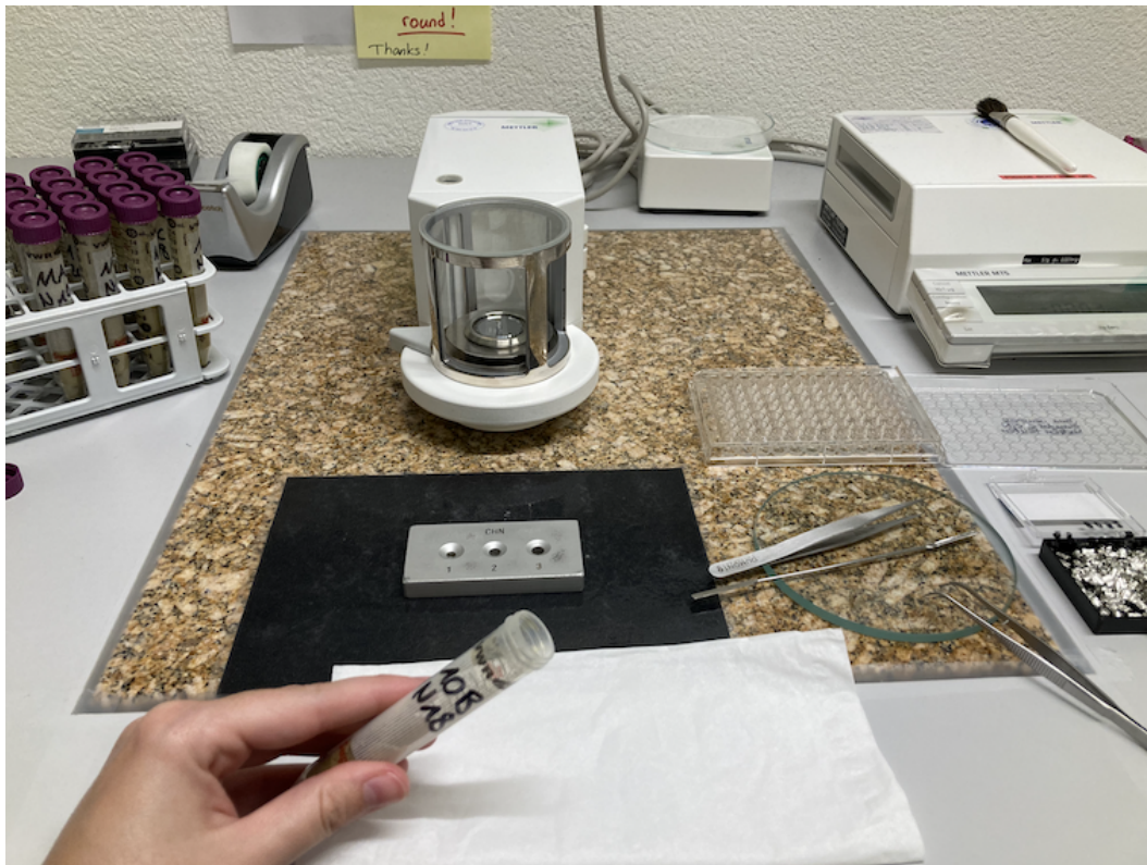
(C) Weighing spruce needle powder in tin capsules
