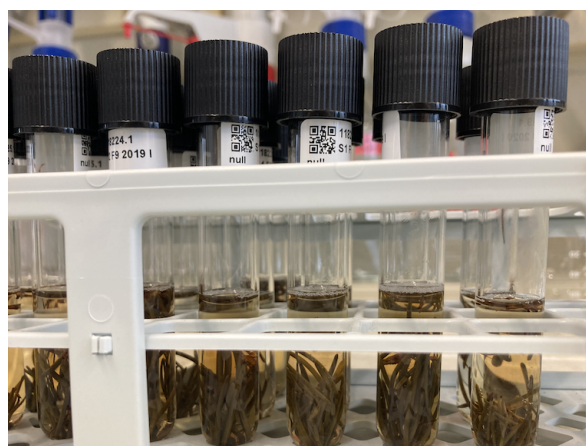
FIGURE 2.11: Acid-base-acid bleaching of Norway spruce ( Picea abies (L.) H.Karst) needles at the Laboratory of Ion Beam Physics, ETH-Zurich
