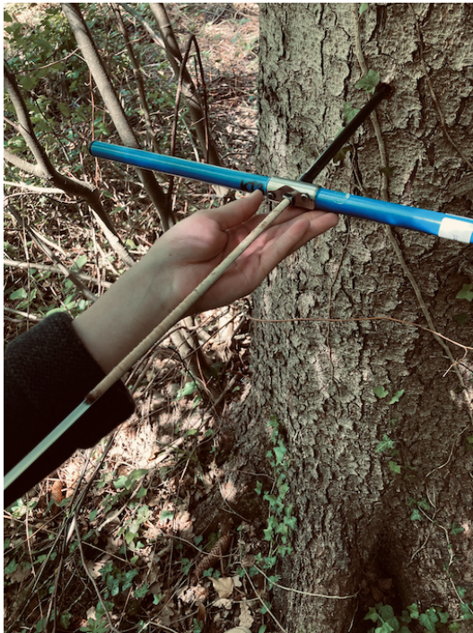
(A) Extracting tree cores with increment corer
