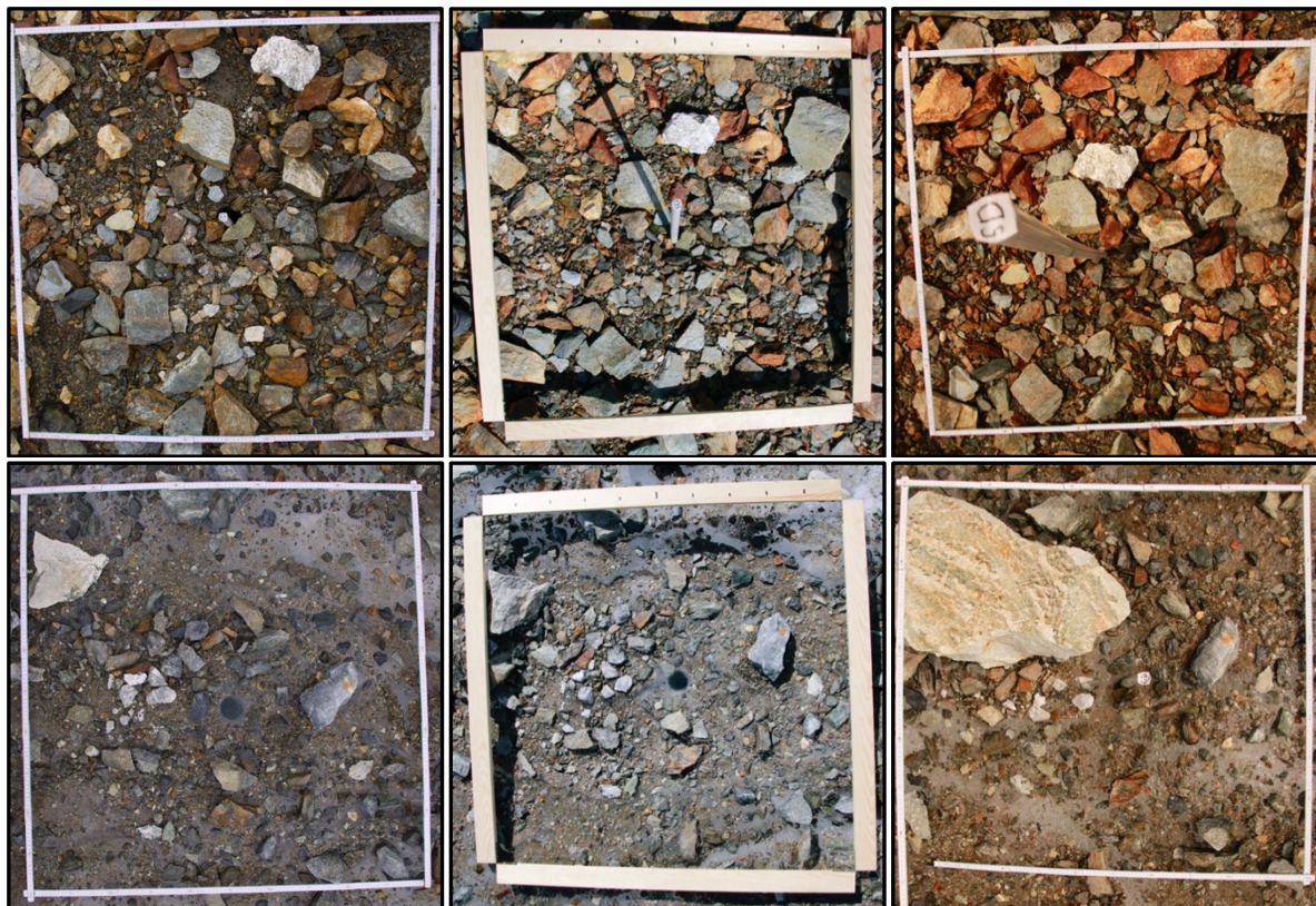
Figure 10. Surface changes between first measurements (12.07.2021) and third measurements (5.08.2021). The upper row of images shows the surface changes for the fully covered surfaces at location 5D, with an overall increase in larger clasts. The lower three images illustrate the changes that occurred on the partially debris covered surface at location 6D.
