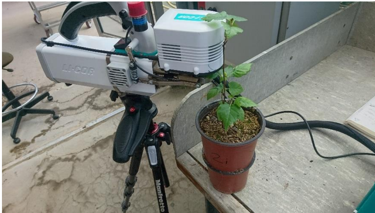
Figure 5: Clamped by the LICOR device, a birch leaf is under investigation to evaluate several physiological leaf properties (stomatal conductance, assimilation rate, transpiration rate)
