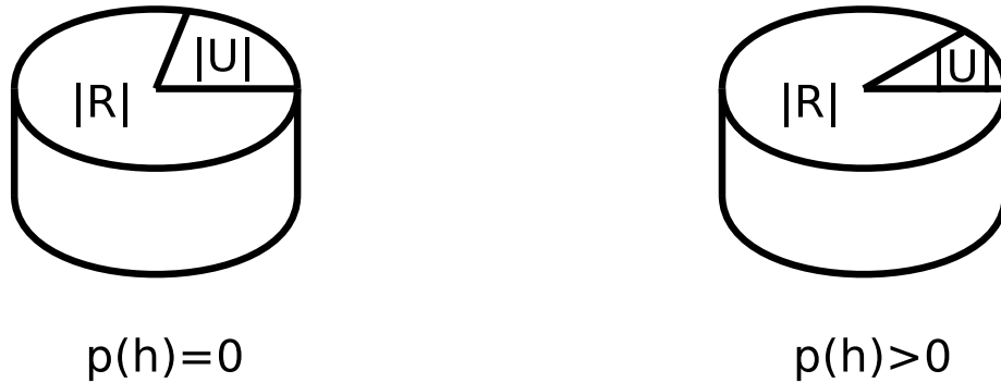
Figure 13: The maximal allowable share of updates for a given redundancy can be determined by solving for p(h) = 0 . The share of updates is smaller if there is overall profit, or p(h) > 0 (assuming same r for all cases).
