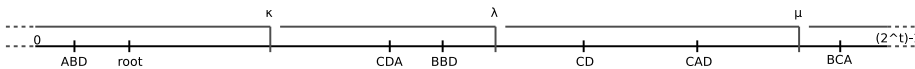
Figure 17: Chord Example: A DHT with three registered nodes \kappa , \lambda and \mu and seven logical elements, the control points ABD, root, BCA, CDA, BBD, CD and CAD. Note that \kappa is responsible for the control point BCA.
