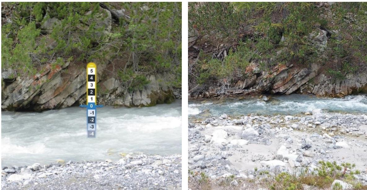
Figure 2: CrowdWater spot at the Ova dal Fuorn in Zernez. Left side: original image with the virtual staff gauge (Simon Meili-Etter, 25.07.17); right side: update for which the water level class -1 was estimated (Mirjam Scheller, 14.09.21).
