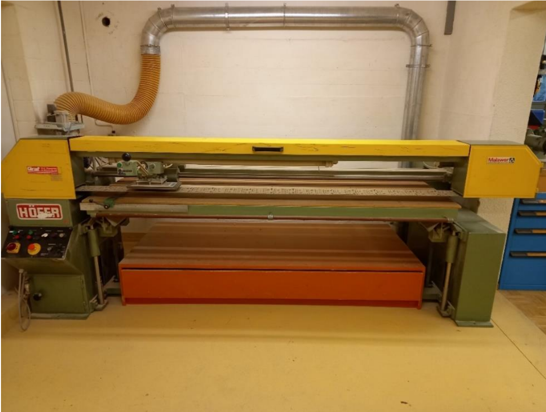
Figure 17 Sanding machine at WSL (Höfer, Graf Maschinen & Service GmbH). The machine allows to sand both wood cores and cross sections, thanks to its dual function. The upper part of the machine allows the user to sand smaller sections or cores, while the bottom part is equipped with a press which is used to sand larger cross-sections while resting them onto an installed moving table (Mattias Barigazzi).
