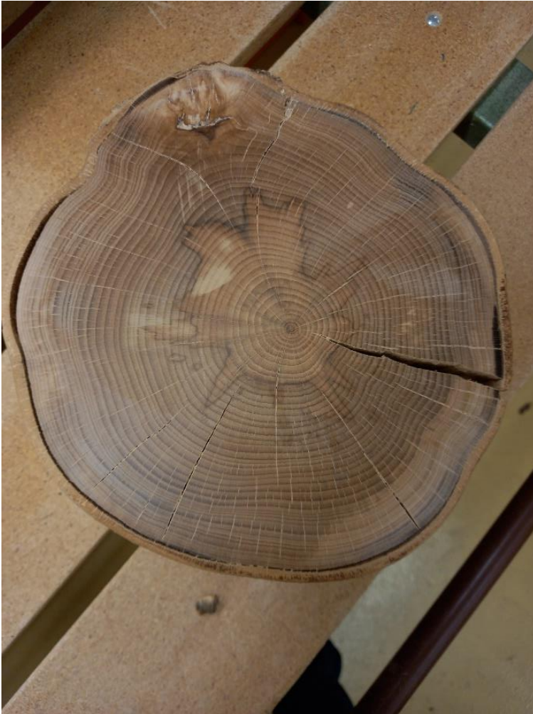
Figure 18 Sample F1_22m after being sanded. The sanding process was achieved by repeatedly scratching the surface of the sample, using different sized sanding paper each time. The result is a cross section with very smooth surface, where each annual ring is clearly visible by the naked eye. In some cases, there are a few burn marks on the surface caused by prolonged contact with the sanding paper and the wood; those are not problematic for the type of analysis that will be conducted (Mattias Barigazzi).
