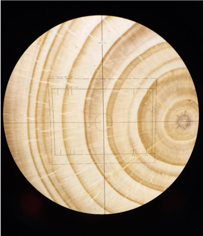
Figure 9 Sample P3_24m analyzed through a binocular with viewfinder. The darker borders represent latewood, while the lighter regions are the earlywood. To measure ring width of an annual ring one must trace the region between two latewood borders using the viewfinder (CC Mattias Barigazzi).
