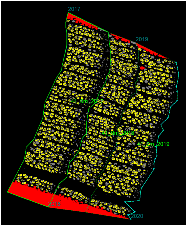
Figure 23 Sample F1_0m (41_0m old name shown in the image) analyzed using the WinCell software. The cells highlighted in yellow are the ones considered good enough to be measured. The gray colored cells are the ones that do not enter in the criteria to be considered good enough cells. There are either too small or broken. The red regions represent the area deemed to be too big to be considered cells. Usually, those areas correspond to either resin canals or big breaks in the sample (Mattias Barigazzi)
