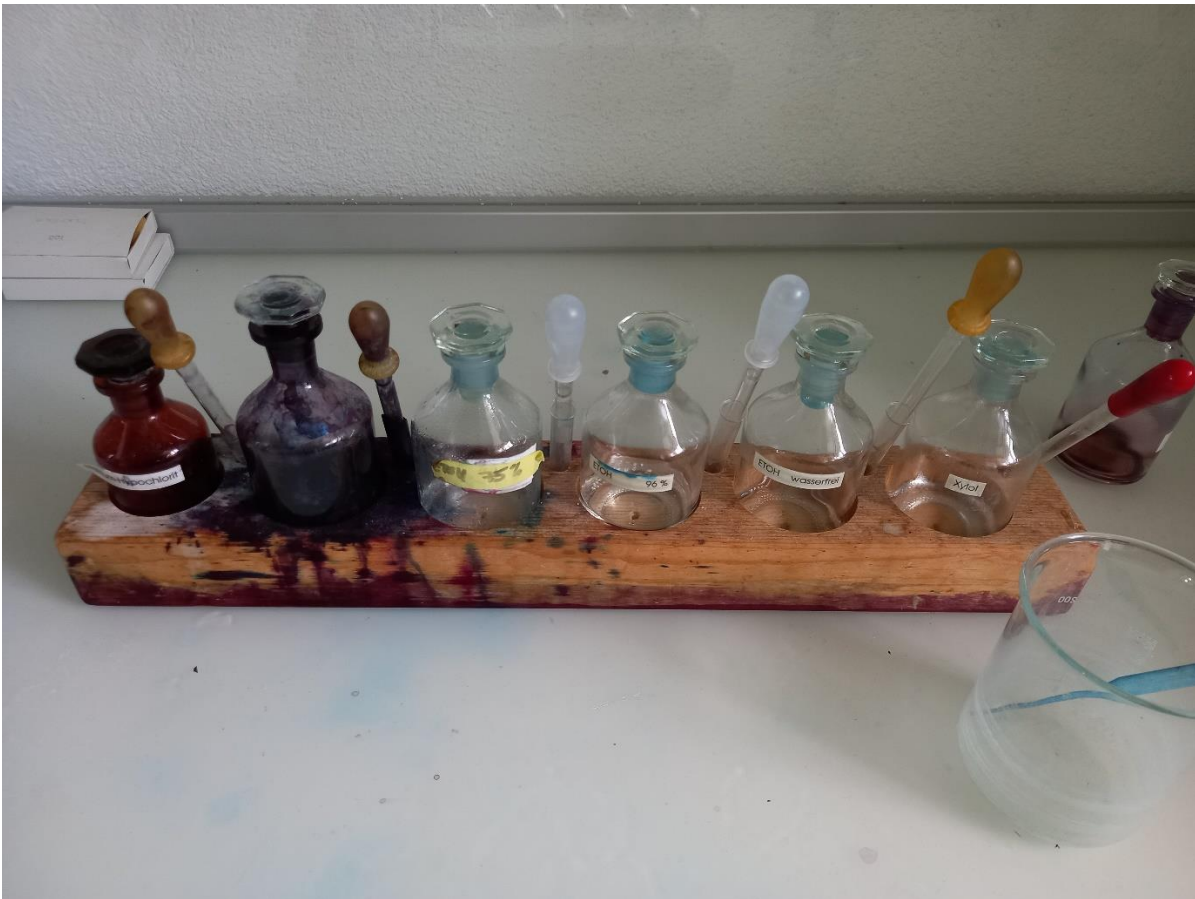
Figure 21 Series of solutions used for the staining process of the thesis. From left to right the solutions are safranin (the staining agent), ethanol (75%), ethanol (96%), ethanol (100%), and xylol. The bigger beaker contains tap water to rinse the solutions off the samples. The left-most bottle of sodium hypochlorite was not used for this kind of staining process (Mattias Barigazzi).
