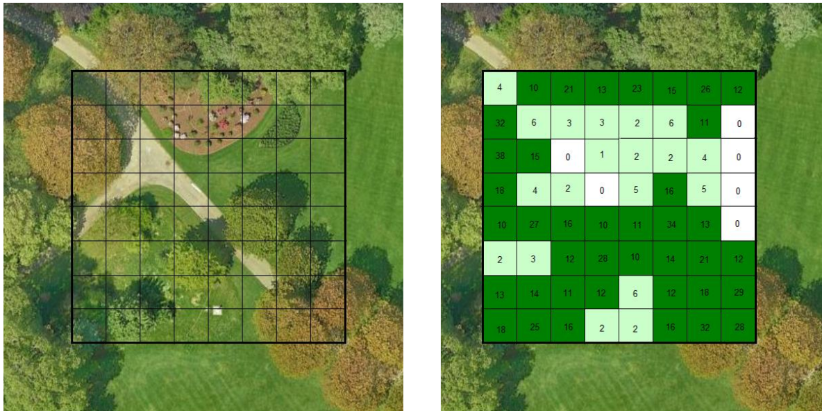
Figure 4. 6. Process of rasterisation of vegetation horizontal density. The number in the grid cell indicates the first return LiDAR points. The value of light green grid cells is below the threshold and therefore is considered non-vegetated.
