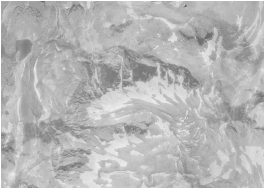
Figure 3.3. Orthophoto mosaic of the year 1961 created by Pix4D software. The representation of the rock glacier in this image is inaccurate as it is somehow split in half and twisted.
