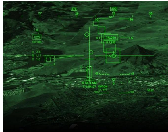
Figure 8 Augmented Night Vision Sight of a F-35 Helmet. From Mola (2017).
