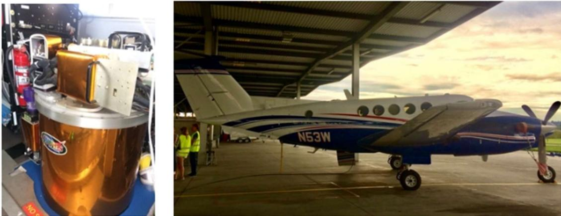
FIGURE 3.1. The AVIRIS-NG spectrometer developed by NASA/JPL (left) and its airborne platform being used; the “Super King Air” research aircraft (right) [29].
