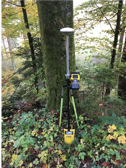
FIGURE 3.4. Trimble R7 GNSS used for the collection of ground reference data.
