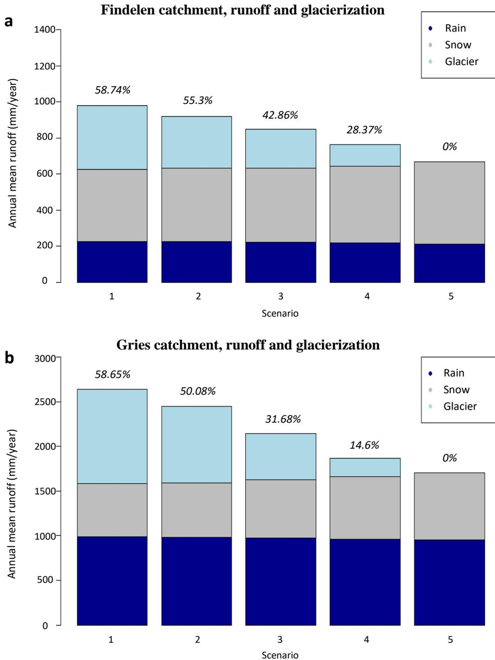
Figure 19: Representation of the three main components of simulated runoff: rain, snow and glacier melt. Mean daily runoff is indicated for both Findelen (a) and Gries (b) catchments. The percentage of glacierization is shown on the top of each barplot in both cases.
