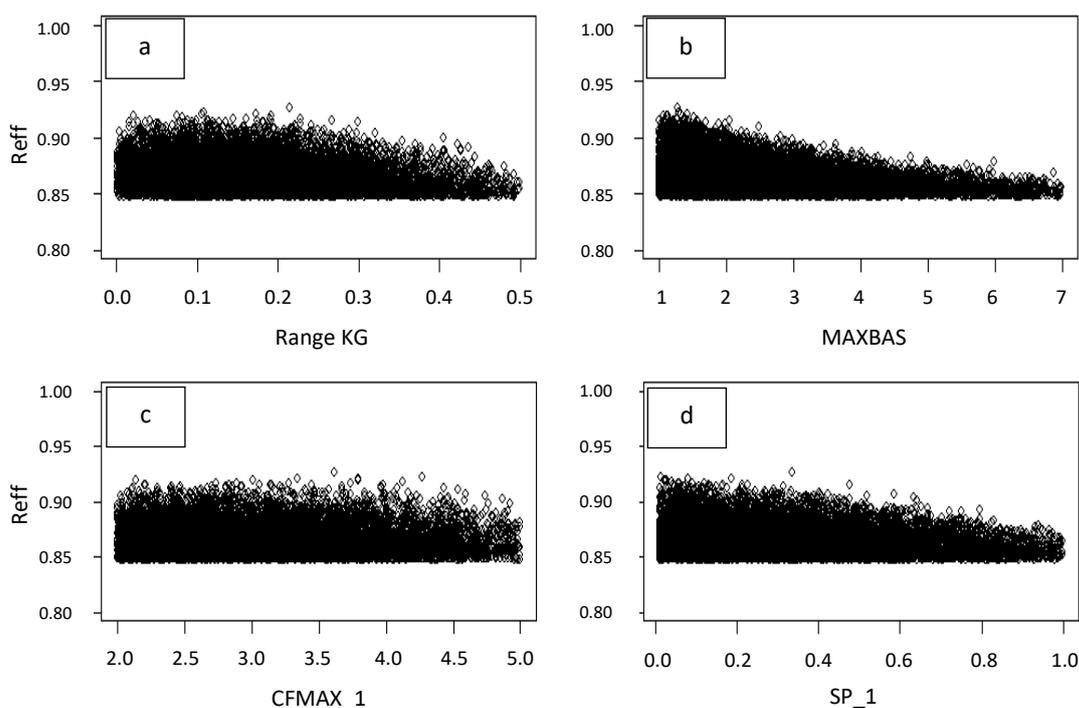
Figure 21: Parameters of the HBV model which show the highest contribution to model efficiency according to the outcomes of the sensitivity analysis which has been performed on the Monte-Carlo automated calibration procedure. On the y-axes, the value of the Nash-Sutcliffe coefficient („ $Reff^*$ “) is represented.
