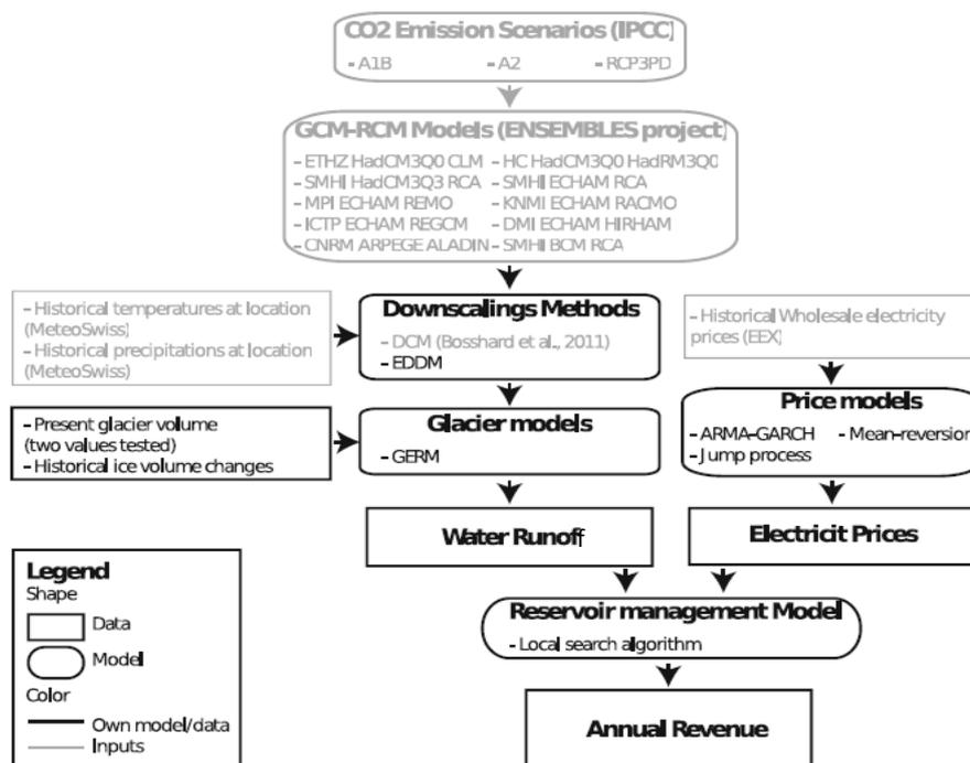
Figure 1: Components and elements of the integrated approach for hydropower production in the specific case of annual income determination. This approach can be applied to quantify the evolution of the produced hydropower energy in the future (Gaudard *et al.*, 2016).
