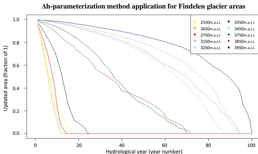
Figure 7: Application of the  $\Delta h$ -parameterization method by Huss *et al.* (2010) for the dynamic glacier routine of the HBV model. The x-axis indicates years, while the y-axis is related to the areal fraction of 1.
