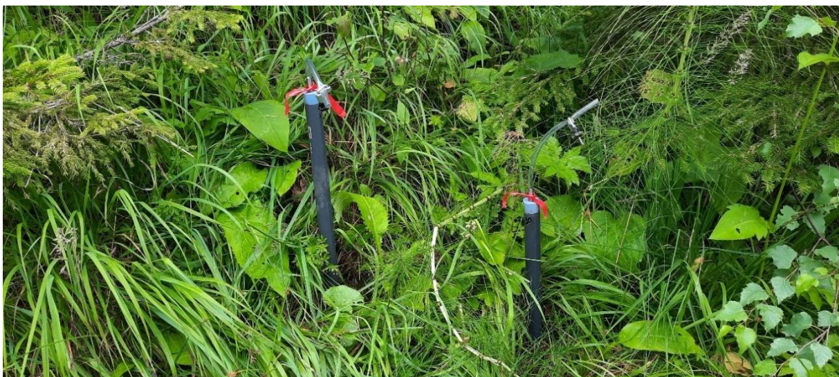
Figure 4.3: Lysimeters L20 and L30 installed at plot 21.3
