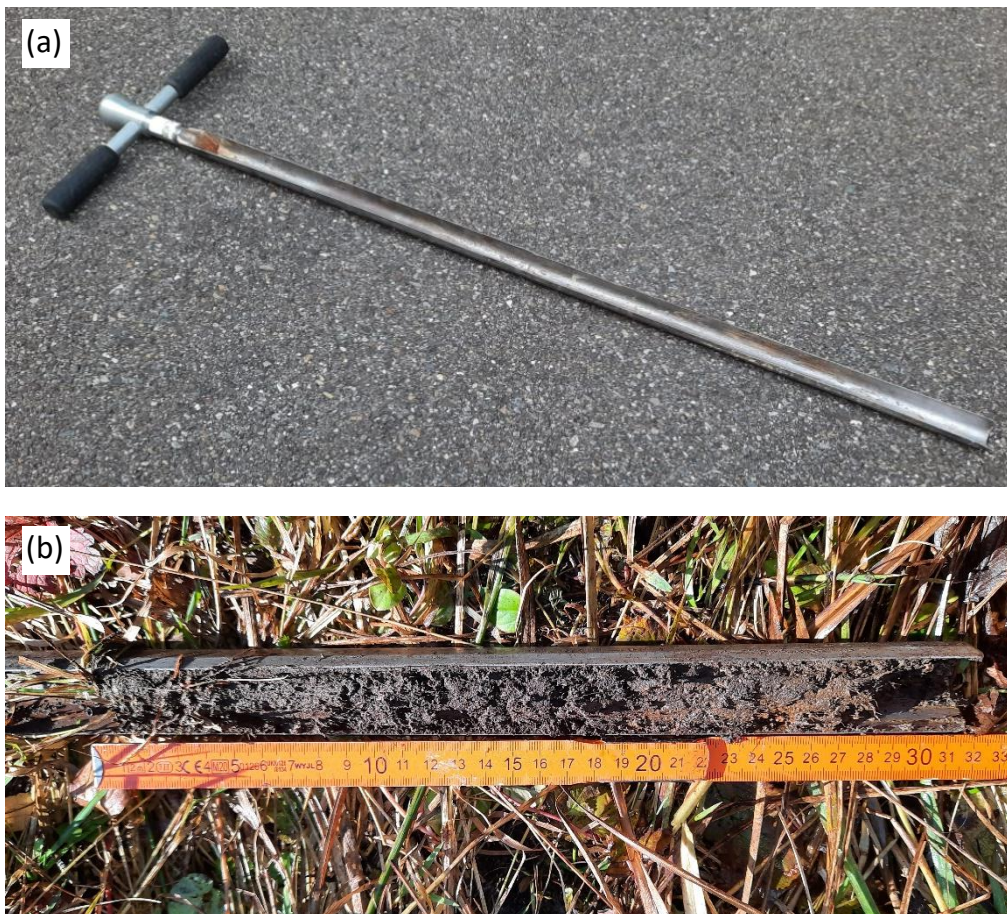
Figure 4.5: (a) Auger used to install lysimeters and take soil samples and (b) soil sample that was divided into three depth sections.
