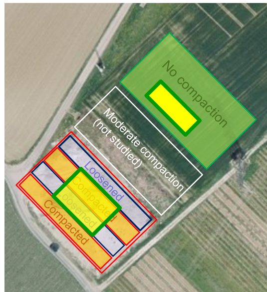
FIGURE 2.4: Sampling location and field classification in compacted , loosened , and uncompacted plots (Johannes et al., 2021a).
