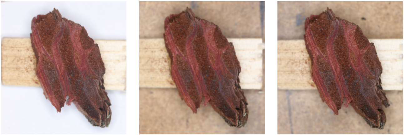
Fig. 8: Example of a plane cut bark sample. On the left is the picture of the bark prior to the treatment, in the middle the sample after 30 minutes of exposure, and on the right the sample after 60 minutes of exposure (Silja Holdener, 2022).
