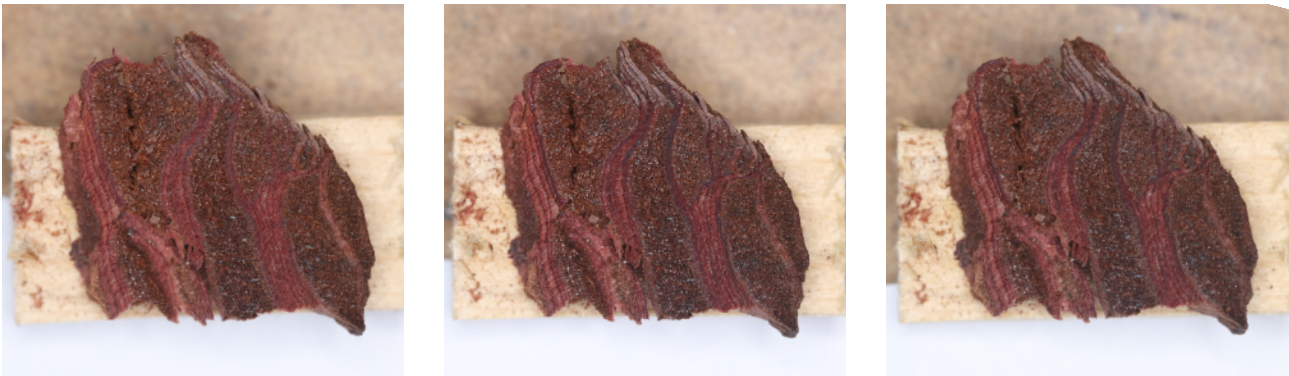
Fig. 7: Example of a plane cut bark sample. On the left is the picture of the bark prior to the treatment, in the middle the sample after three hours of exposure, and on the right the sample after six hours of exposure (Silja Holdener, 2022).
