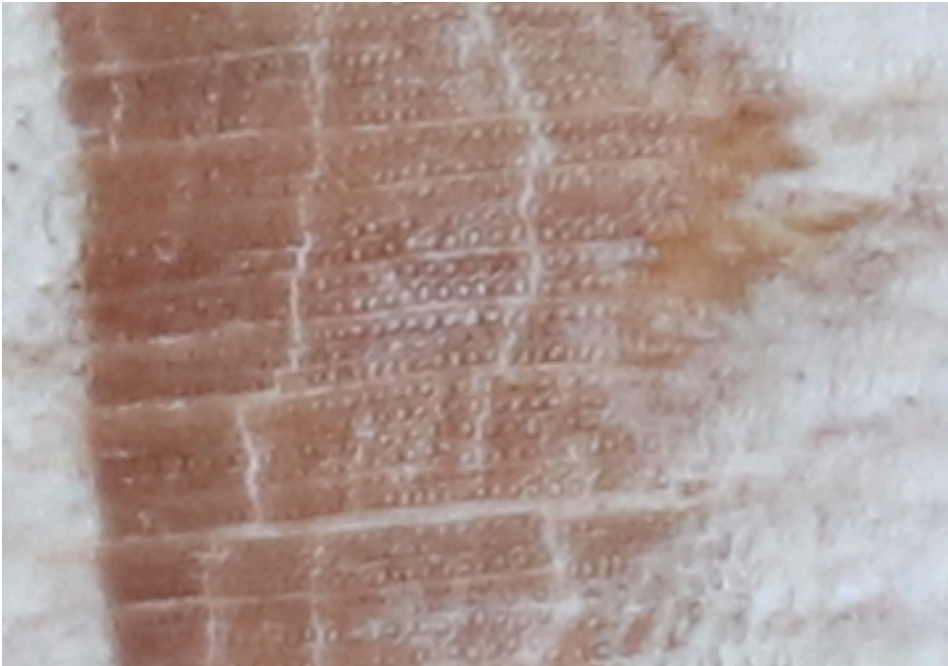
Fig. 3 A: Sample Control 2G showing extreme RW. The cell walls are very thick and a lot of space between the cells is visible (Silja Holdenr, 2022).
