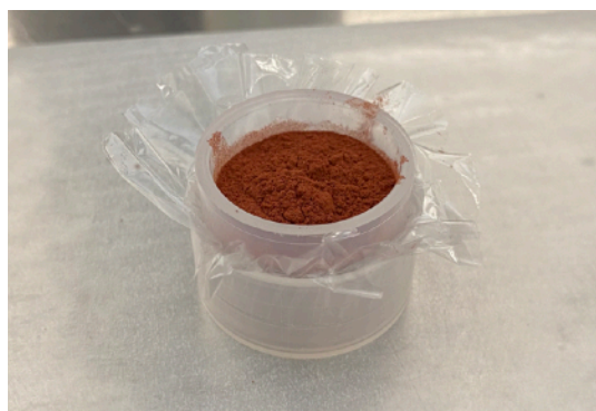
Fig. 9: Finely ground bark powder filled into a sample cup for XRF measurements (Silja Holdener, 2022).
