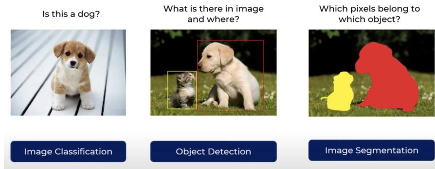
Figure 2.2: Three main tasks of CV deep learning. *Image Classification*: The model learns to classify an image, *Object Detection*: The model learns to detect in what region of an image specific items are located, *Image Segmentation*: The model learns to perform a pixel-wise classification. (Graphic: Patel 2020)
