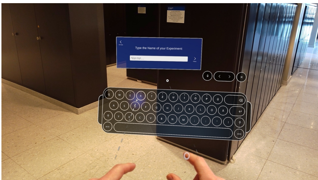
Figure 22: Dialogue to create a new experiment with the holographic keyboard to type a name.
