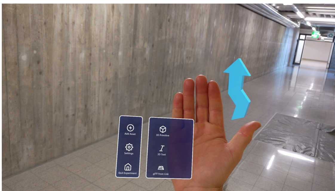
Figure 34: The submenus in the hand menu are sometimes blocked if users access it with their right hand.
