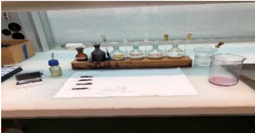
Figure 17: Set up for dying. From left to right Canada balsam, bleach dye, ethanol solutions, xylol and water.
