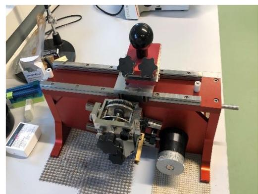
Figure 16: Lab-microtome for cutting micro sections.
