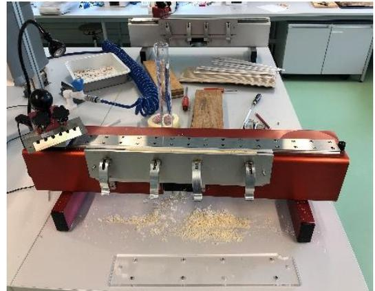
Figure 14: Sample prepared for cutting on core microtome.
