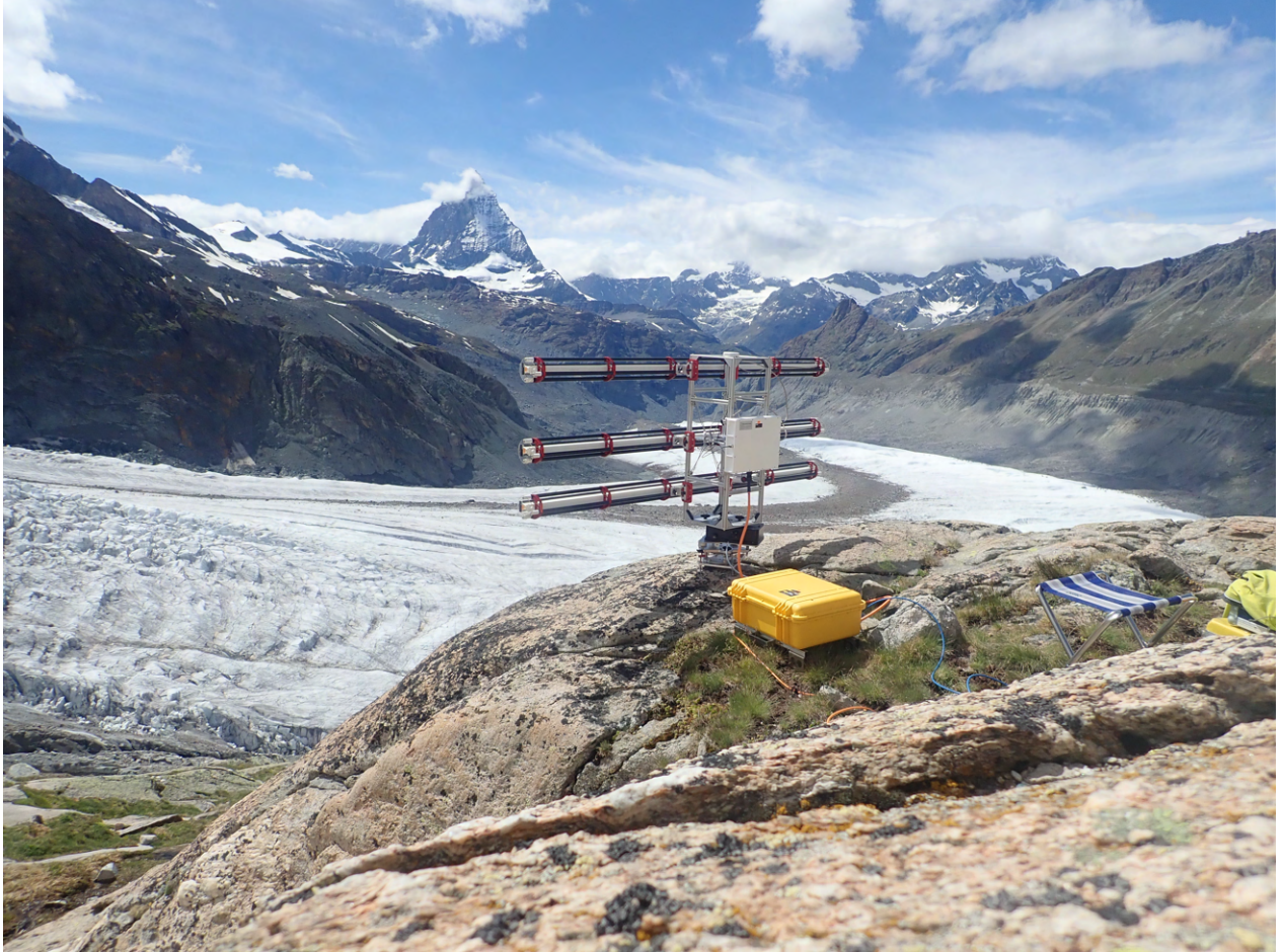
Figure 3: GAMMA Portable Radar Interferometer installed above Gorner Glacier
