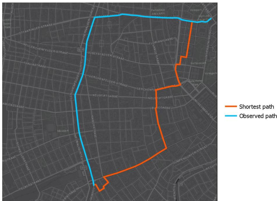
Figure 11: Example of an observed trip with fewer turns than the associated shortest distance path.
