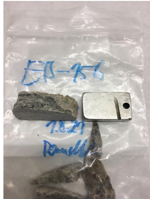
Figure 10: Broken handpieces of EB-200 during sawing. Figure 11: Biggest handpiece of EB-156 during sawing, next to the model of the required size of a thin section block.
