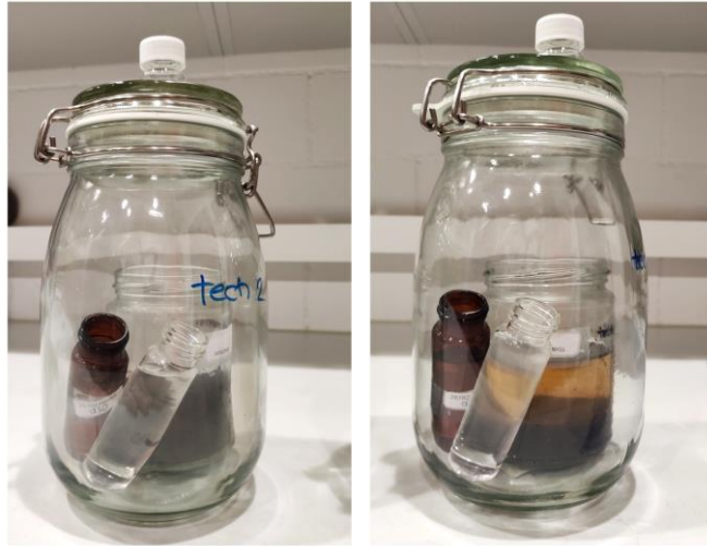
Figure 1: The final set-up. On the left side, the field moist treatment and on the right side, the saturated treatment. Brown vials with the NaOH solution and clear vials with water.
