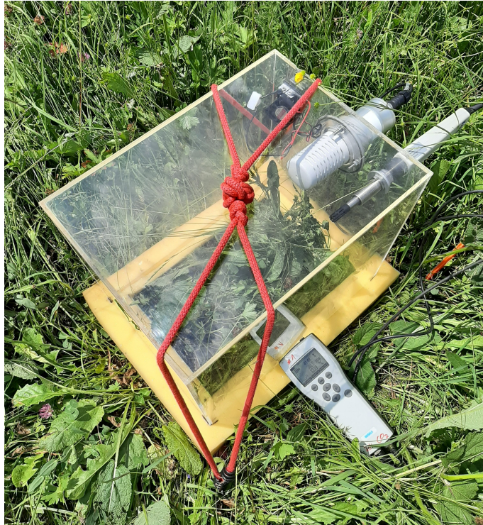
Figure 8: Ecosystem CO_2 gas exchange measurements technique. In the photo, the transparent cuvette can be seen, fixed to the ground with the red rubber band (secured to the ground with metal stakes) and yellow cell foam band. The humidity and air temperature sensor inside the chamber, the infrared CO_2 probe and the small fan can be seen, in order from the right. Leaning against the cuvette is also the logger, connected to the sensors. The thermometer recording the ground temperature at the time of measurement is not visible.
