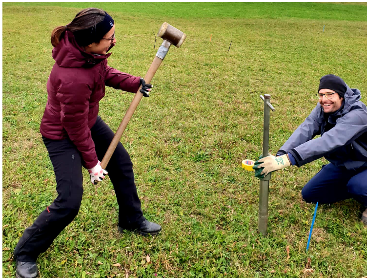
Figure 25: Soil sampling (01.11.2022), with Robin Giger in the picture, using sampling tubes to collect probes with a defined volume.
