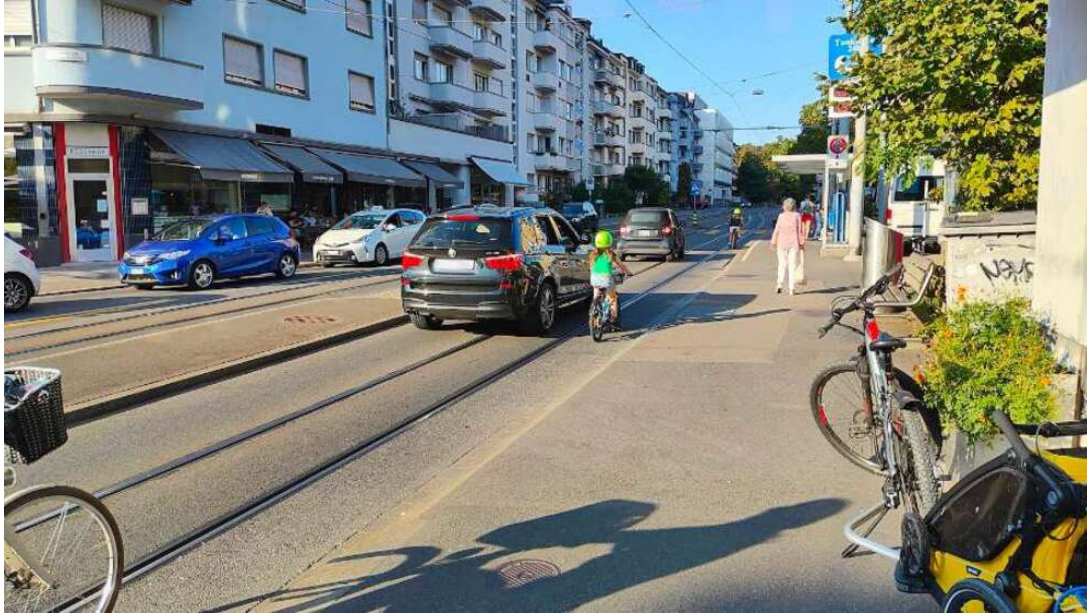
Figure 4.5: Tram station with dangerous tram tracks, high curbs and narrow road width. Source: bikeable.ch, user: stefanhaustein
