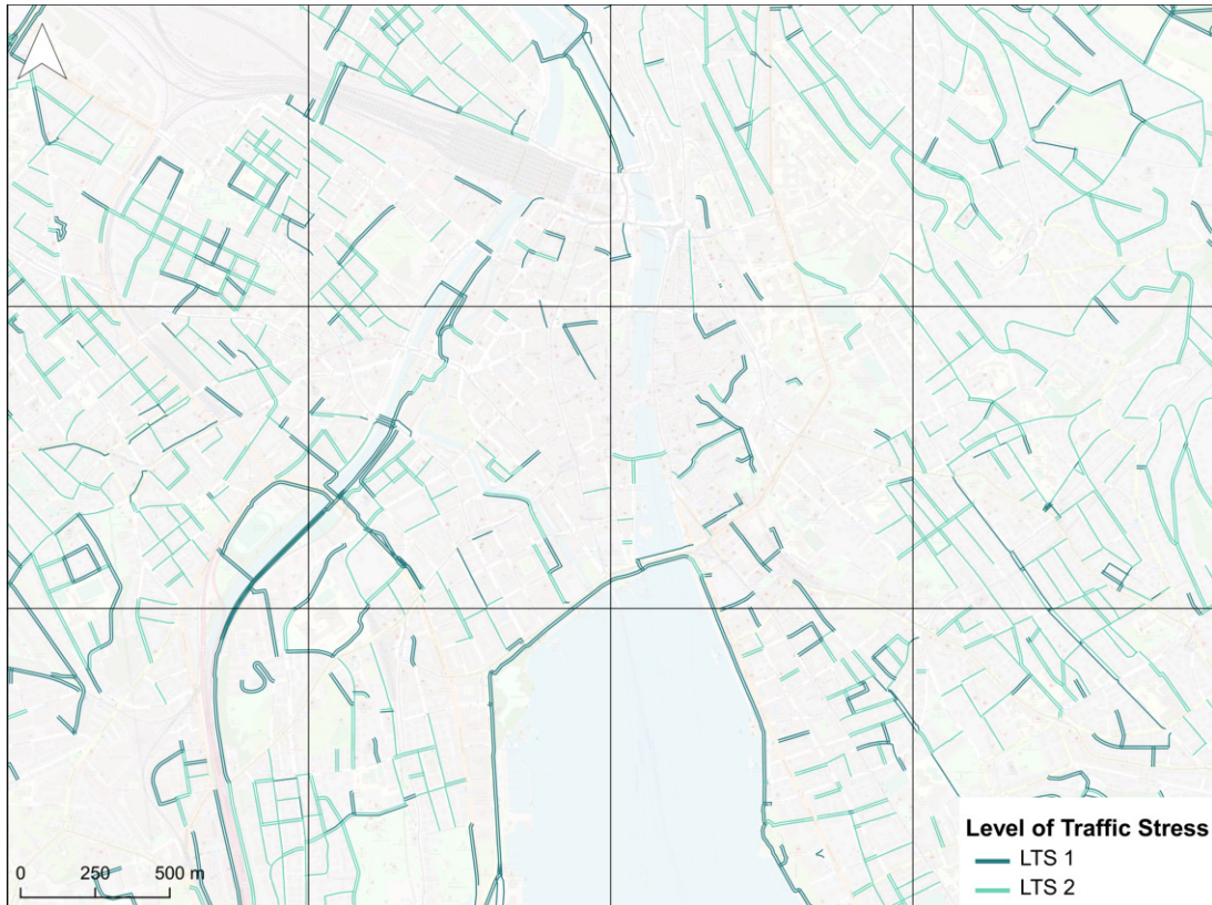
Figure 5.4: Network for the level of traffic stress group 2, section from city centre
