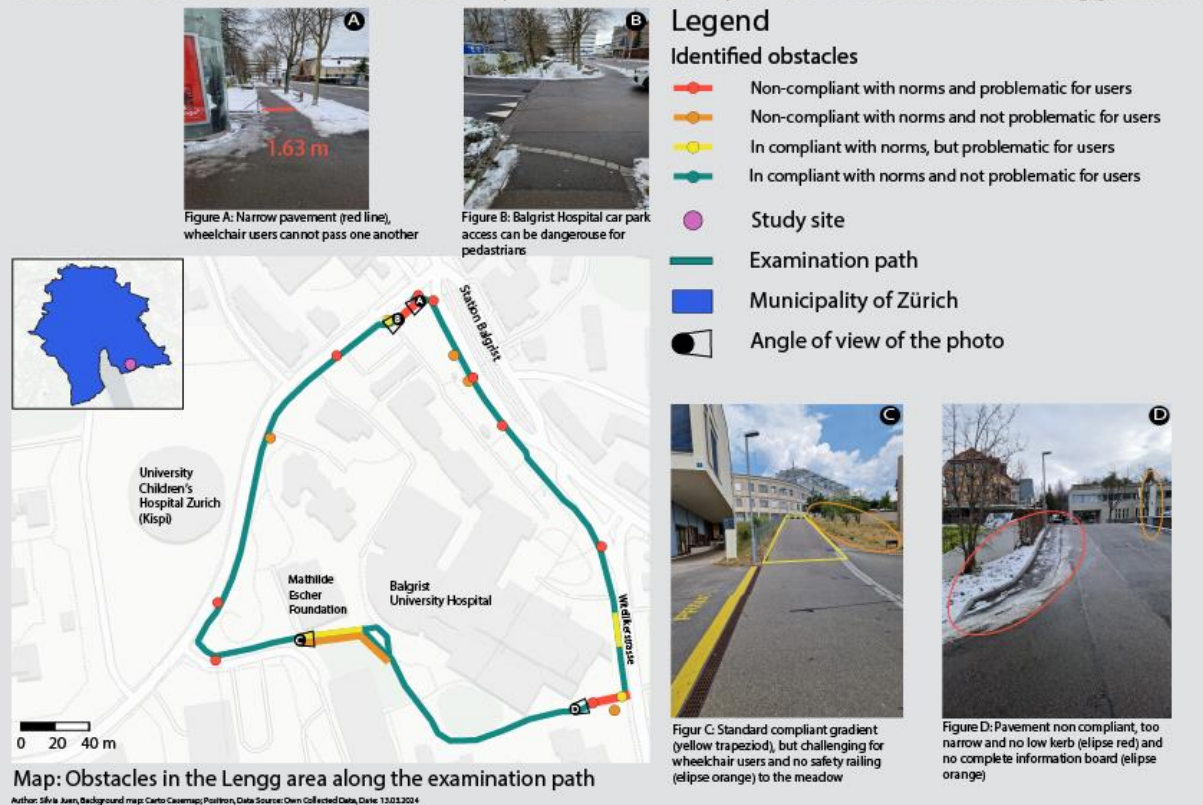
Figure 30: Map of obstacles for wheelchair users on the examination route (in petrol) in the Lengg Healthcare Area in Zurich (Created by Silvia Juen).
