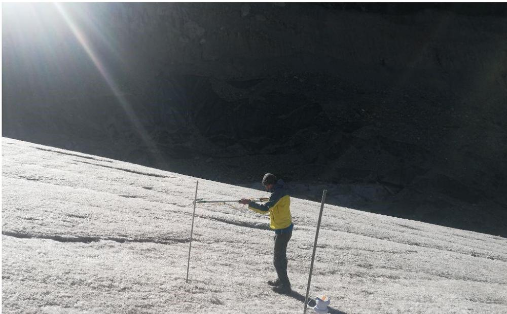
Figure 6: Measurements with the handheld albedometer. Photo by Anna Czerniejewska (20.09.2022, 16:11).
