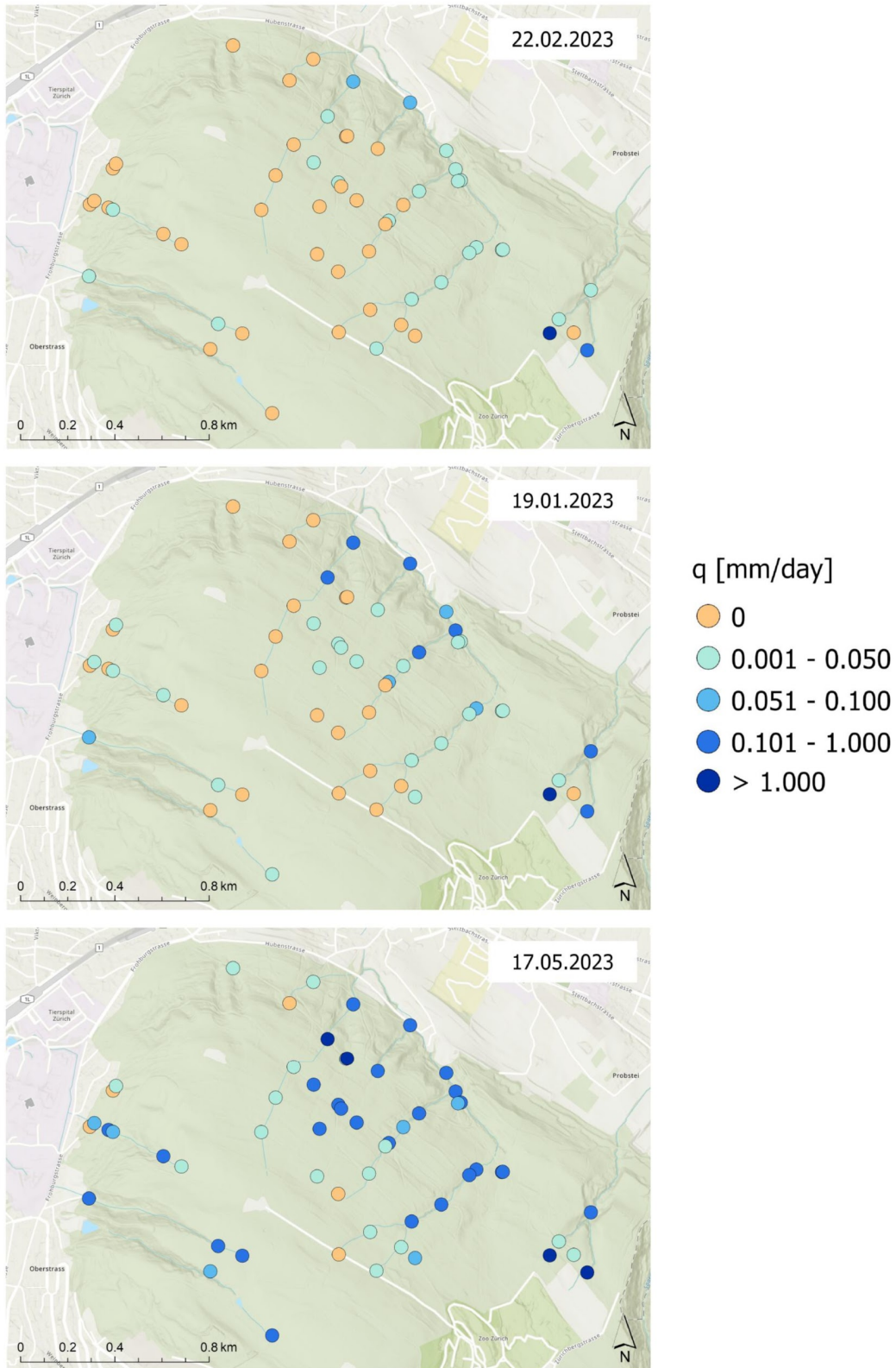
Figure 11: Specific discharge ( q ) on three selected days. Top: Measurements during the day of lowest cumulative discharge (February 22, 2023). Middle: Day of median cumulative discharge (January 19, 2023). Bottom: Highest cumulative discharge per day (May 17, 2023). For the maps for all other survey dates, see Figure A1 - A4 in Appendix A3
