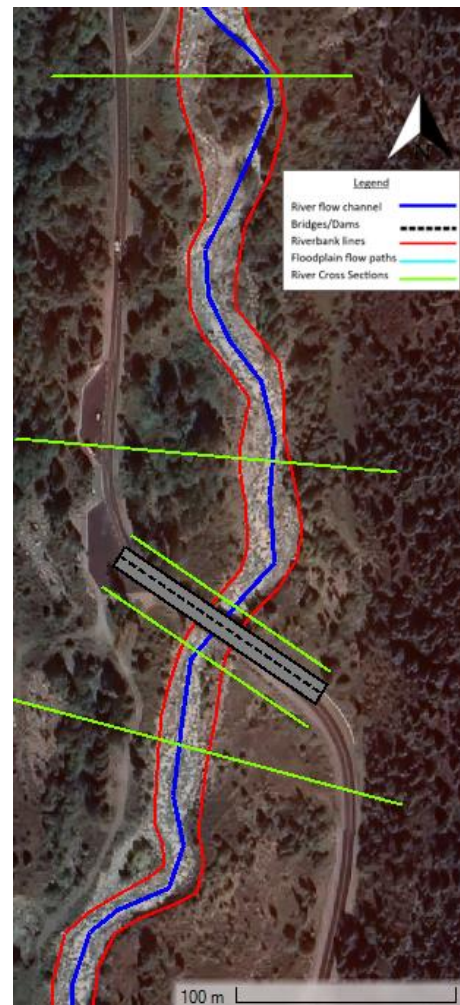
Figure 12: HEC-RAS geometry visualization of national park bridge.
